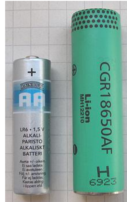
AA cell vs 18650 Lithium cell ~12Wh energy, ~49g
